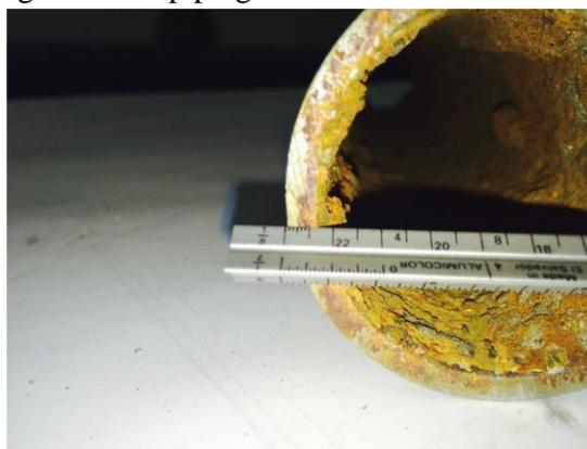
Sample 1: Visible Corrosion & Deteriorated Wall Thickness
